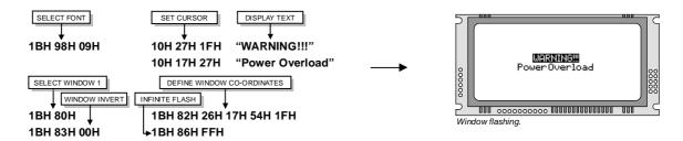
The window mode can be changed to 'clear' for a flash on/off effect.
