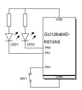
With asynchronous communications enabled, the status of PA0-PA7 can be transmitted when a change in level is detected on any pin. This automatic response mode can be enabled by using the 'UART SETUP' command. When this mode is enabled, the VFD module can reliably check port changes every 15ms. With auto send disabled (default) a manual read command is required to determine the port status.
