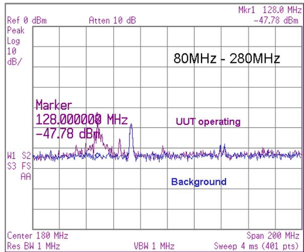
Peak at 153MHz is local interference (ship-to-shore), not associated with operation of Module under test.
