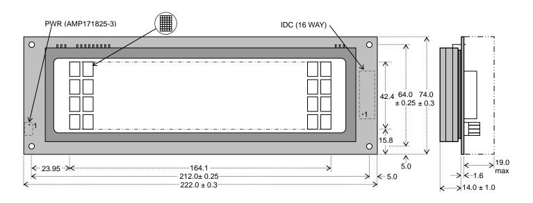
Dimensions in mm & subject to tolerances. Mounting holes 3.5mm dia.
