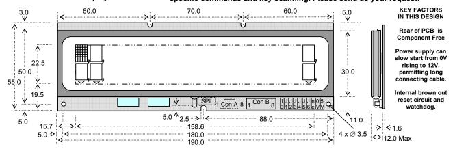
Con B is Molex 90814-0008 which mates with Molex 90327-0308. The 5V outputs on the jumper pads are for 15mA slave logic connection.
