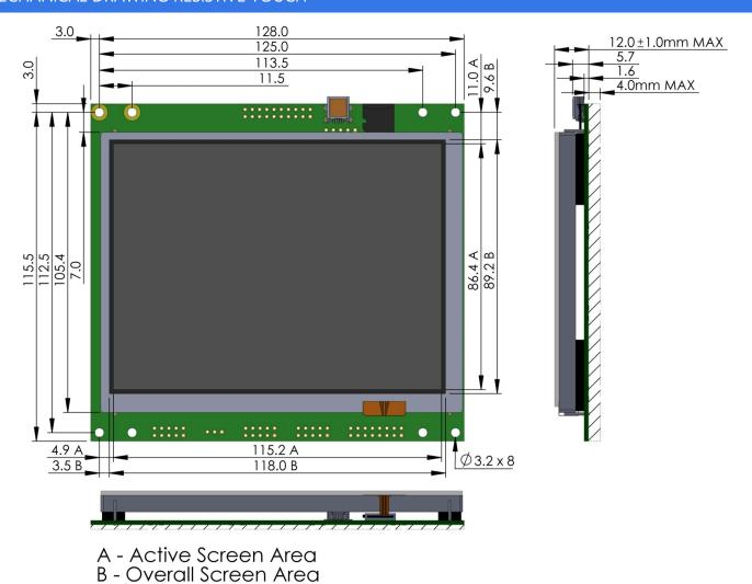
Figure 3 – TU640x480C-K61XA1RU Mechanical drawing. Reference dimensions only.
