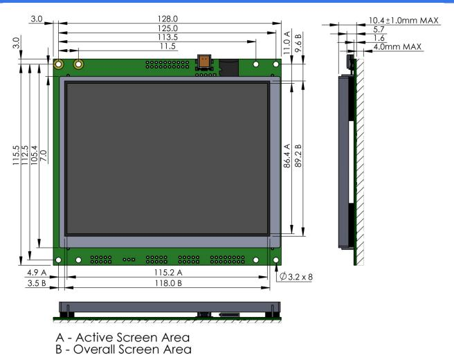
Figure 4 – TU640x480C-K61XA1NU Mechanical drawing. Reference dimensions only.
