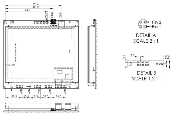
Figure 5 - TU640x480C-K61XA1XX Connector Location drawing. Reference dimensions only. Note: RU and NU connector locations are the same as the image above.
