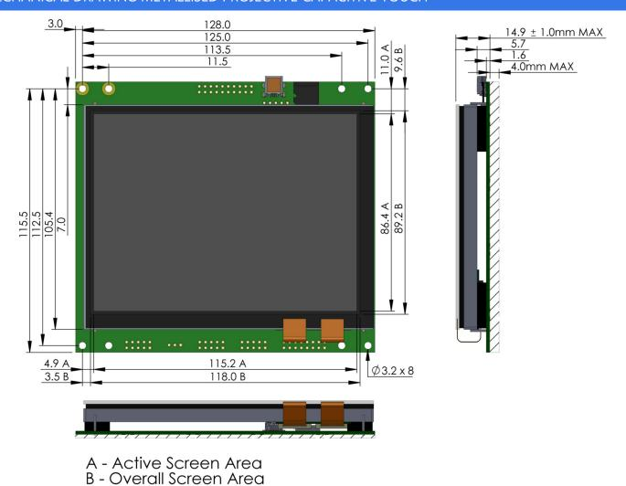
Figure 2 – TU640x480C-K61XA1MU Mechanical drawing. Reference dimensions only.
