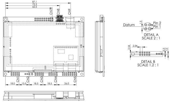
Figure 5 - TU480x272C-K61XA1XX Connector Location drawing. Reference dimensions only. Note: RU and NU connector locations are the same as the image above.
