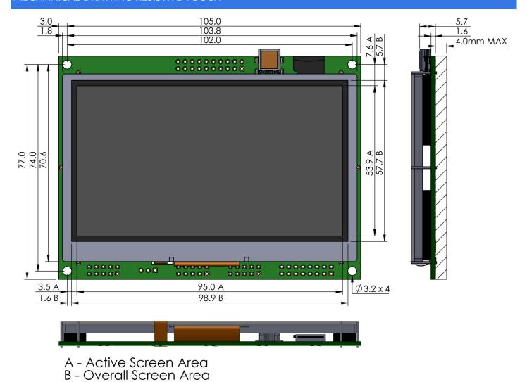
Figure 3 - TU480x272C-K61XA1RU Mechanical drawing. Reference dimensions only.
