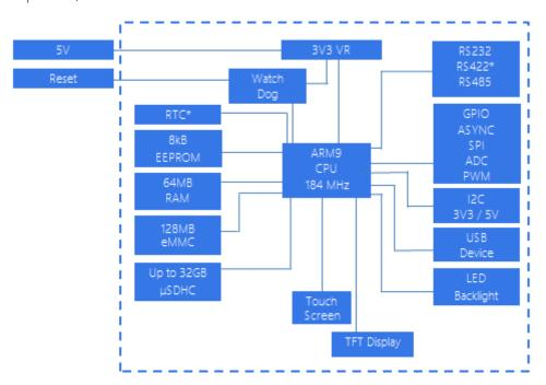
Figure 1 - Circuit Block Diagram. \* Optional.
