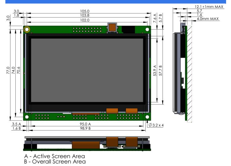
Figure 2 – TU480x272C-K61XA1MU Mechanical drawing. Reference dimensions only.
