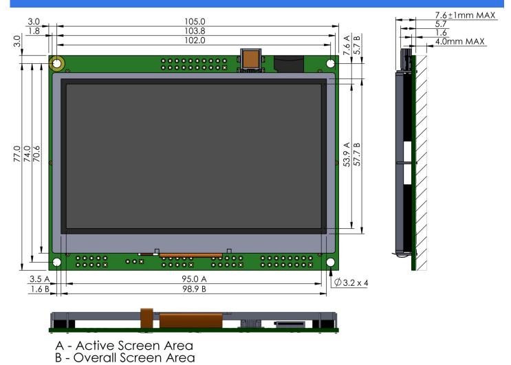
Figure 4 – TU480x272C-K61XA1NU Mechanical drawing. Reference dimensions only.
