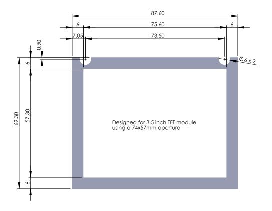
Note: All dimensions are in millimeters unless otherwise stated. Scale 1:1
